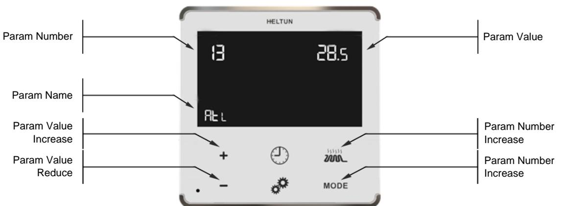
To scroll through the menu, press or hold the Heating Element
