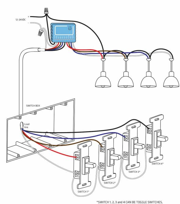
\*SWITCH 1, 2, 3 and 4 CAN BE TOGGLE SWITCHES, MOMENTARY SWITCHES OR TOGGLE WITH MEMORY SWITCHES. YOU MUST SET THE PARAMETERS TO THE RIGHT VALUE FOR DIFFERENT TYPES OF SWITCHES.
