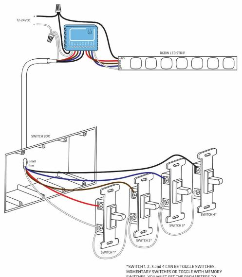
SWITCHES. YOU MUST SET THE PARAMETERS TO THE RIGHT VALUE FOR DIFFERENT TYPES OF SWITCHES.
