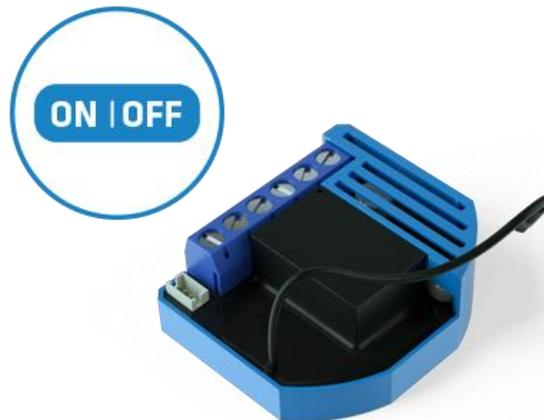
*The Qubino Flush 1D Relay is ideal for remotely controlling one electrical device (door lock, door opener, small appliances, etc.). The output contact is voltage free (dry contact), so different power supply loads can be connected to the Flush 1D Relay.*
